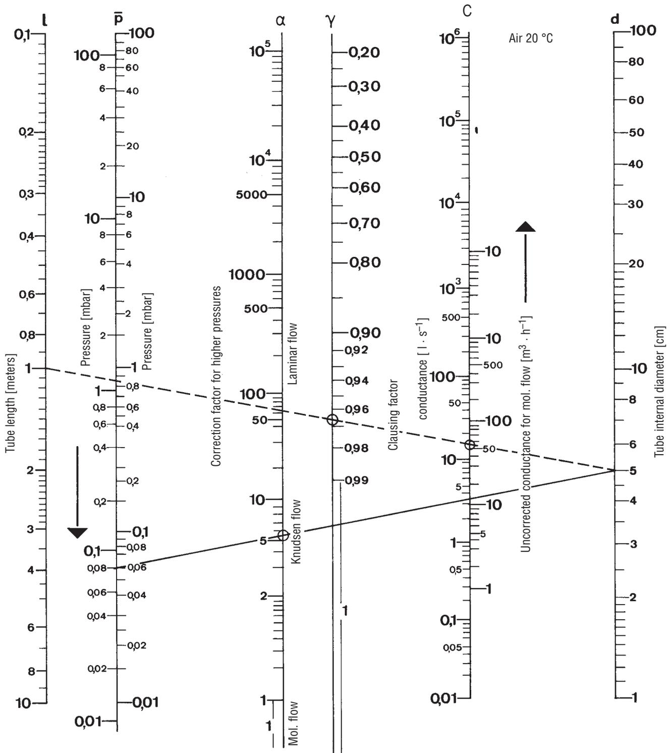
**Procedure:** For a given length ( $l$ ) and internal diameter ( $d$ ), the conductance  $C_m$ , which is independent of pressure, must be determined in the molecular flow region. To find the conductance  $C^*$  in the laminar flow or Knudsen flow region with a given mean pressure of  $p$  in the tube, the conductance value previously calculated for  $C_m$  has to be multiplied by the correction factor  $\alpha$  determined in the nomogram:  $C^* = C_m \cdot \alpha$ .
