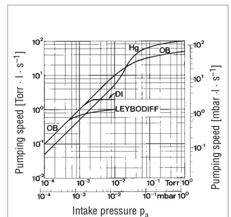
Fig. 2.49 Pumping speed of various vapor pumps (derived from Fig. 2.48)
