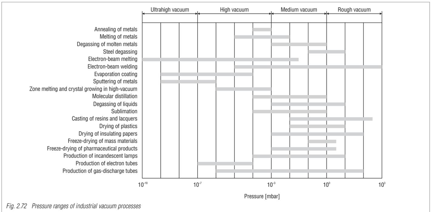
Fig. 2.72 Pressure ranges of industrial vacuum processes
