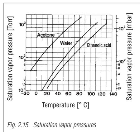
Fig. 2.15 Saturation vapor pressures
