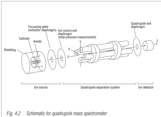
Fig. 4.2 Schematic for quadrupole mass spectrometer
