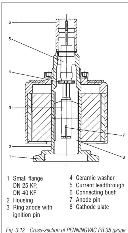
Fig. 3.12 Cross-section of PENNINGVAC PR 35 gauge
