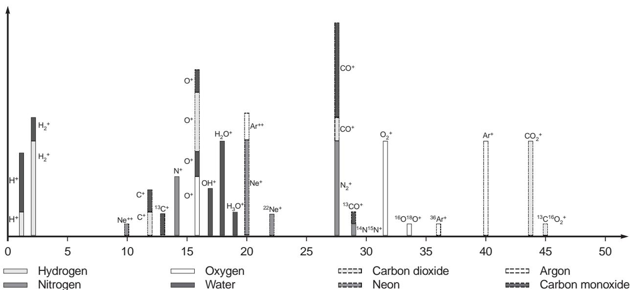
Evaluation problems: The peak at atomic number 16 may, for example, be due to oxygen fragments resulting from  $O_2$ ,  $H_2O$ ,  $CO_2$  and  $CO$ ; the peak at atomic number 28 from contributions by  $N_2$  as well as by  $CO$  and  $CO$  as a fragment of  $CO_2$ ; the peak at atomic number 20 could result from singly ionized Ne and double-ionized Ar
