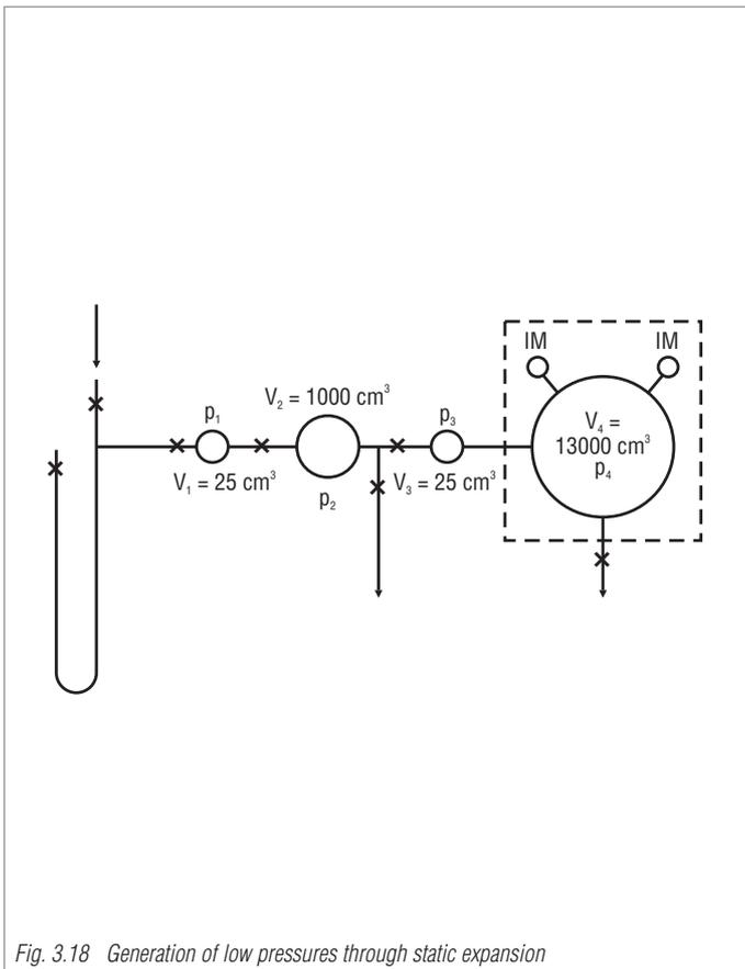
Fig. 3.18 Generation of low pressures through static expansion
