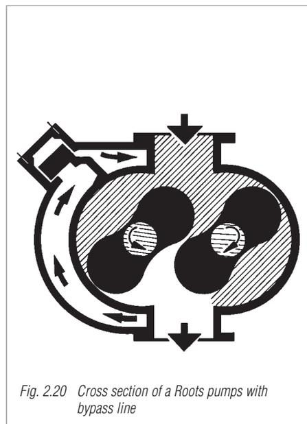
Fig. 2.20 Cross section of a Roots pumps with bypass line
