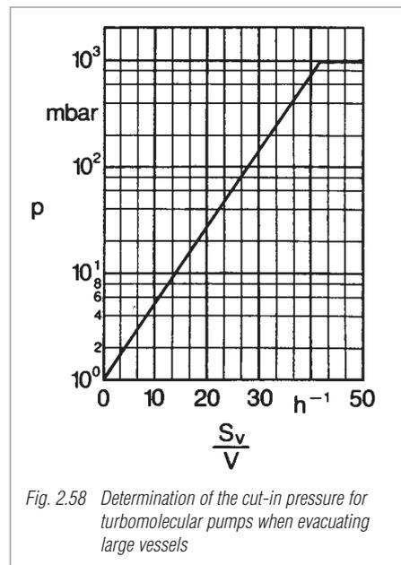
pump sets and large vacuum chambers. At a known pumping speed for the backing pump S<sub>V</sub> (m<sup>3</sup>/h) and a known volume for the vacuum chamber (m<sup>3</sup>) it is possible to estimate the cut-in pressure for the turbomolecular pump:
