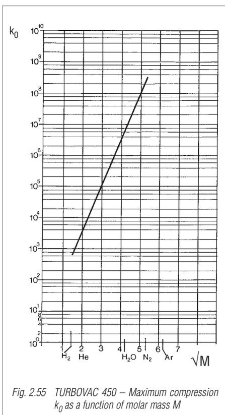
Fig. 2.55 TURBOVAC 450 – Maximum compression  $k_0$  as a function of molar mass  $M$
