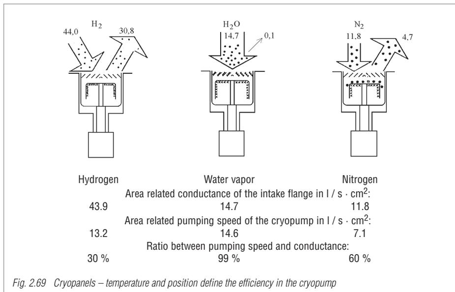
Fig. 2.69 Cryopanel – temperature and position define the efficiency in the cryopump
