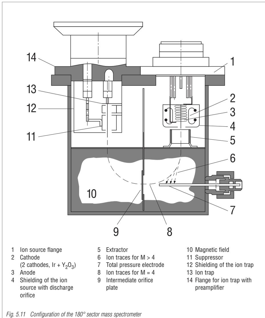
Fig. 5.11 Configuration of the 180° sector mass spectrometer
