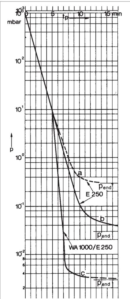
Fig. 2.77 Pumpdown time,  $t_p$ , of a  $5 \text{ m}^3$  vessel using a rotary plunger pump E 250 having a nominal pumping speed of  $250 \text{ m}^3/\text{h}$  with (a) and without (b) gas ballast, as well as Roots/rotary plunger pump combination WA 1001 / E250 for a cut-in pressure of 10 mbar for the WA 1001 (c)
