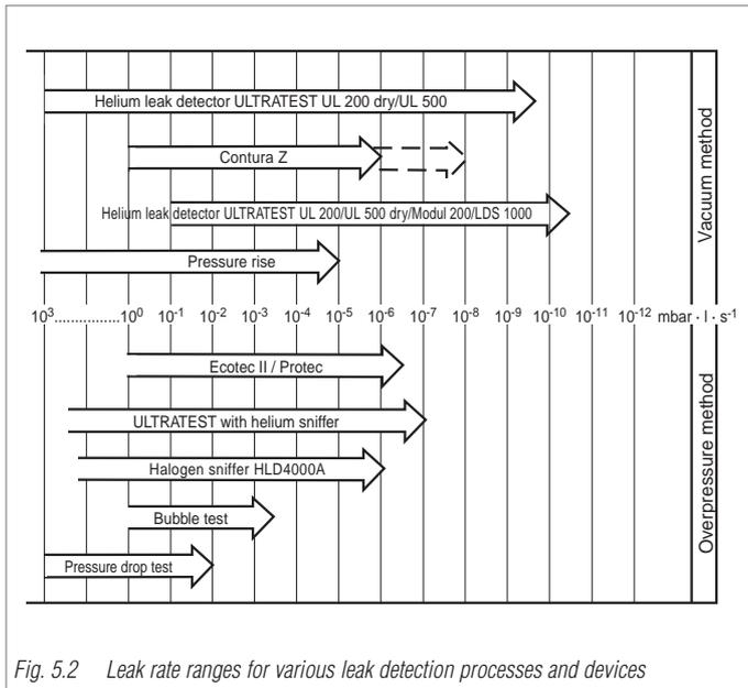
Fig. 5.2 Leak rate ranges for various leak detection processes and devices
