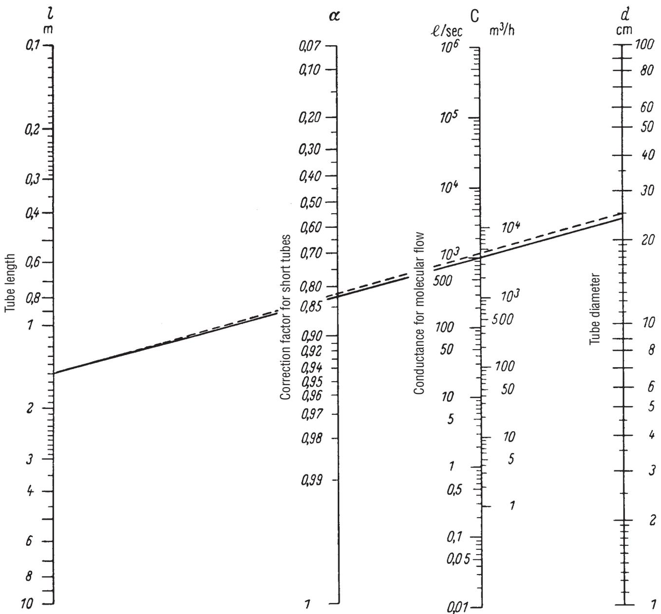
**Example:** What diameter  $d$  must a 1.5-m-long pipe have so that it has a conductance of about  $C = 1000 \text{ l / sec}$  in the region of molecular flow? The points  $l = 1.5 \text{ m}$  and  $C = 1000 \text{ l/sec}$  are joined by a straight line which is extended to intersect the scale for the diameter  $d$ . The value  $d = 24 \text{ cm}$  is obtained. The input conductance of the tube, which depends on the ratio  $d / l$  and must not be neglected in the case of short
