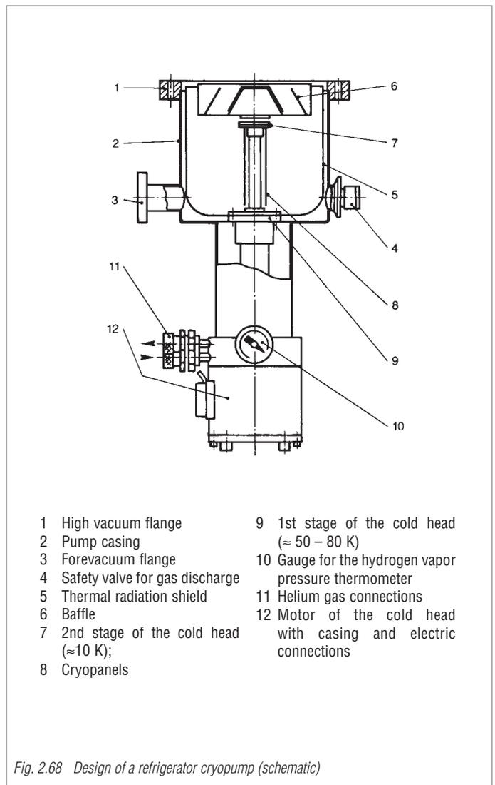
stage (7) of the cold head are coated with activated charcoal on the inside in order to be able to pump gases which do not easily condense and which can only be pumped by cryosorption (see 2.1.9.4).
