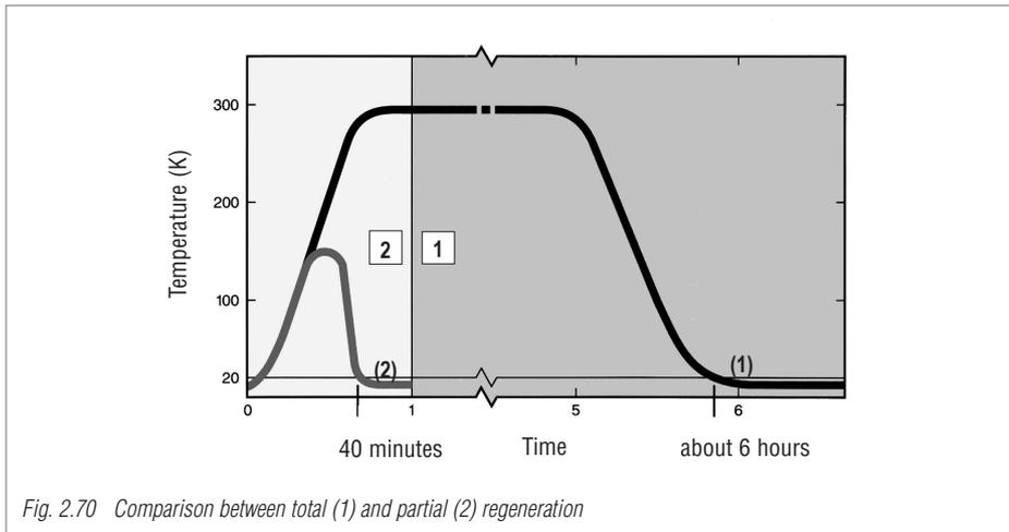
Fig. 2.70 Comparison between total (1) and partial (2) regeneration
