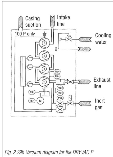
Fig. 2.29b Vacuum diagram for the DRYVAC P
