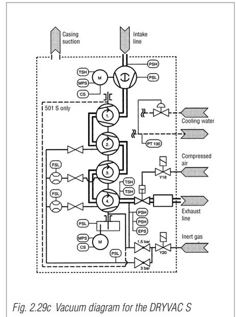
Fig. 2.29c Vacuum diagram for the DRYVAC S
