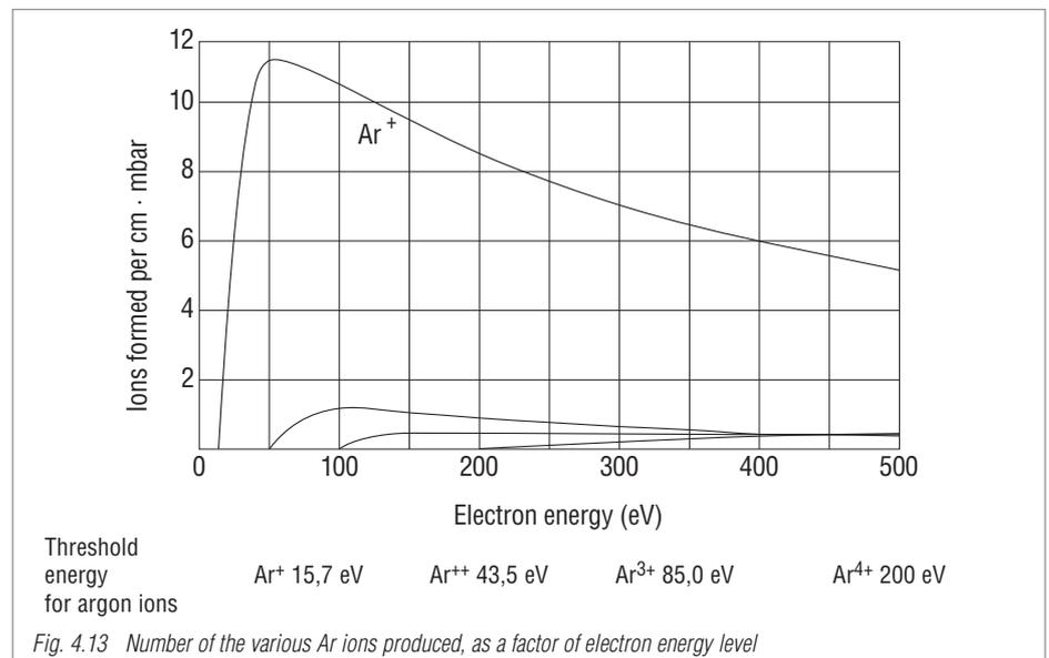
Fig. 4.13 Number of the various Ar ions produced, as a factor of electron energy level
