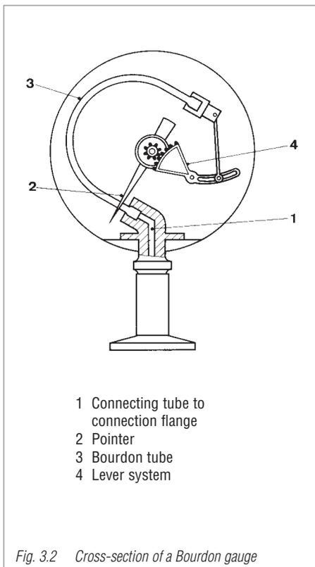
Fig. 3.2 Cross-section of a Bourdon gauge
