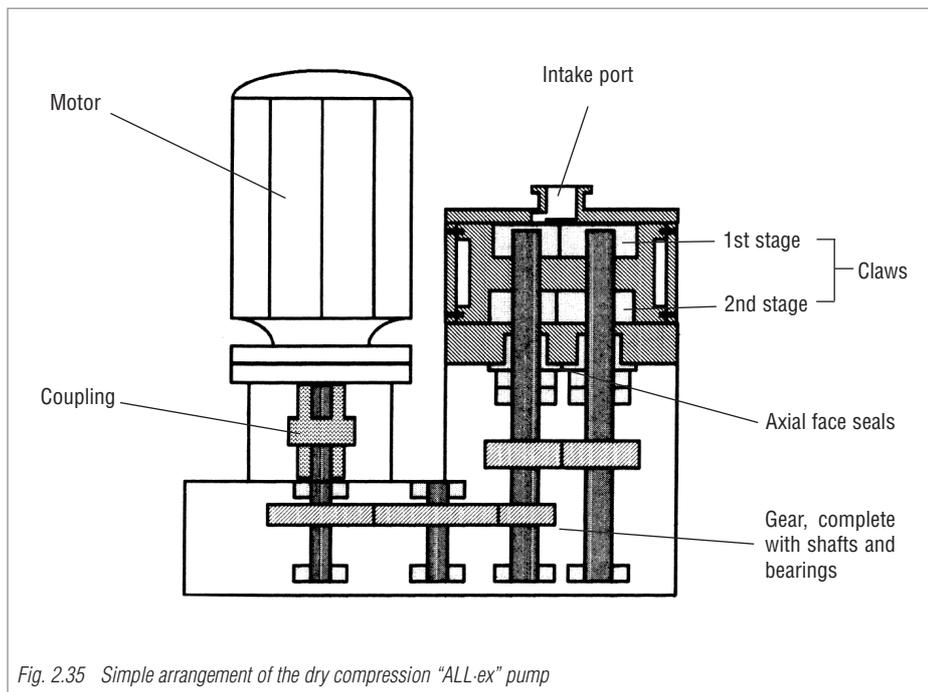
Fig. 2.35 Simple arrangement of the dry compression "ALL-ex" pump
