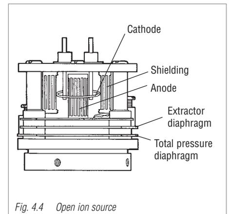
Fig. 4.4 Open ion source
