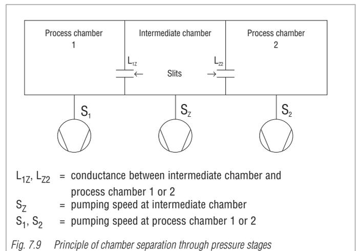
The transport arm cycles one station further after each process step and in this way transports the substrates from one process station to the next. During cycling all processes are switched off and the stations are vacuum-linked to each other. As soon as the arm has reached the process position, the individual stations are sepe-
