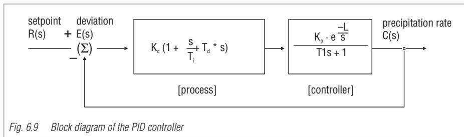
Fig. 6.9 Block diagram of the PID controller
