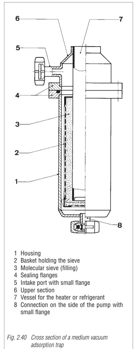
Fig. 2.40 Cross section of a medium vacuum adsorption trap
