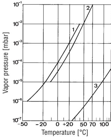
1 NBR (Perbunan) 2 Silicone rubber 3 Teflon
