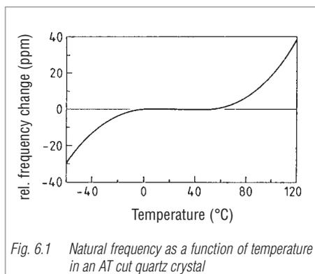
Fig. 6.1 Natural frequency as a function of temperature in an AT cut quartz crystal
