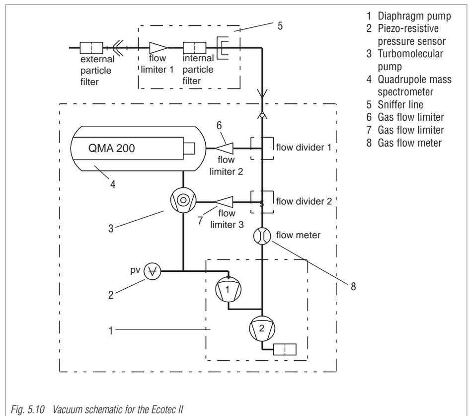
Fig. 5.10 Vacuum schematic for the Ecotec II
