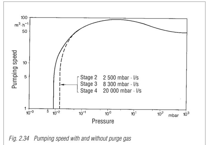
Fig. 2.34 Pumping speed with and without purge gas
