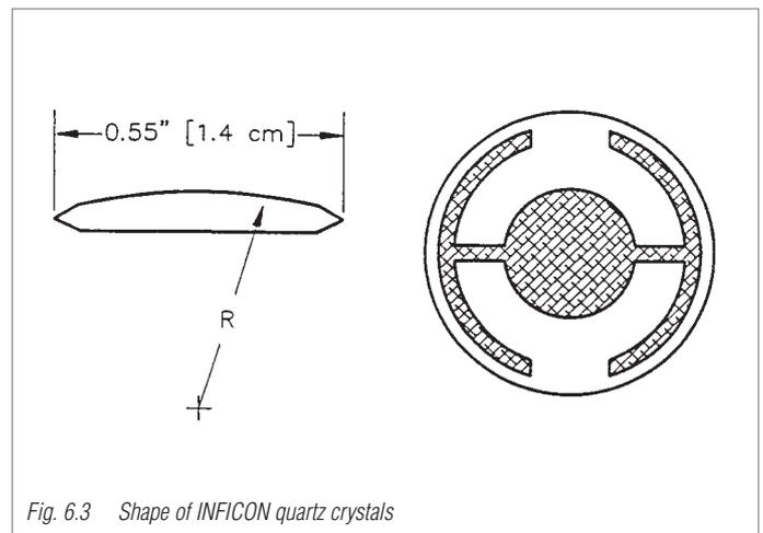
Fig. 6.3 Shape of INFICON quartz crystals
