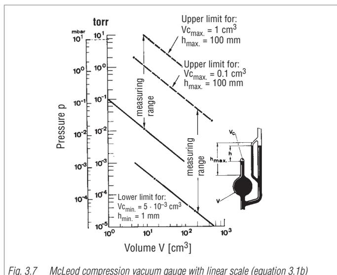
Fig. 3.7 McLeod compression vacuum gauge with linear scale (equation 3.1b)
