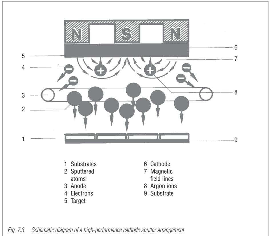
Fig. 7.3 Schematic diagram of a high-performance cathode sputter arrangement
