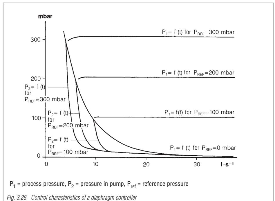
$P_1$  = process pressure,  $P_2$  = pressure in pump,  $P_{ref}$  = reference pressure
