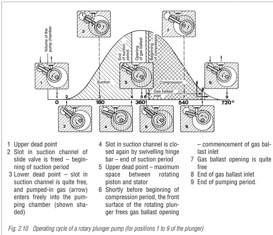
Fig. 2.10 Operating cycle of a rotary plunger pump (for positions 1 to 9 of the plunger)
