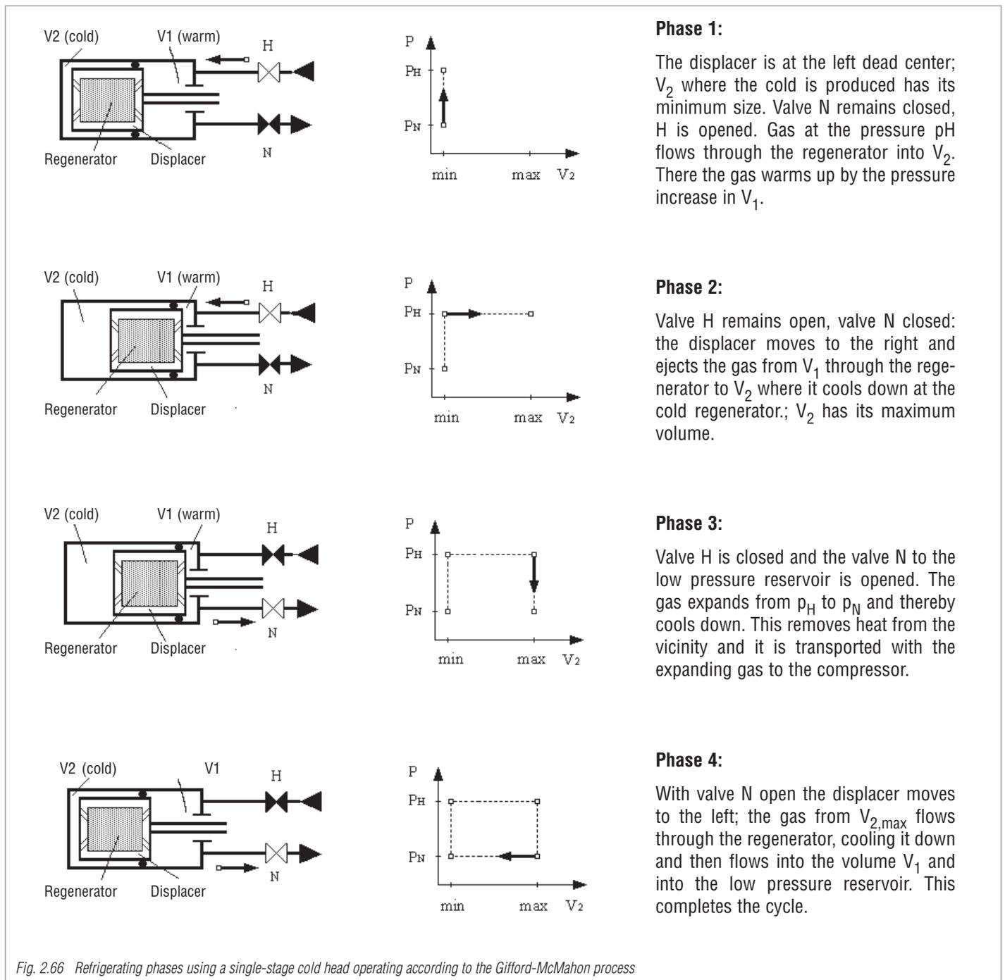
Fig. 2.66 Refrigerating phases using a single-stage cold head operating according to the Gifford-McMahon process
