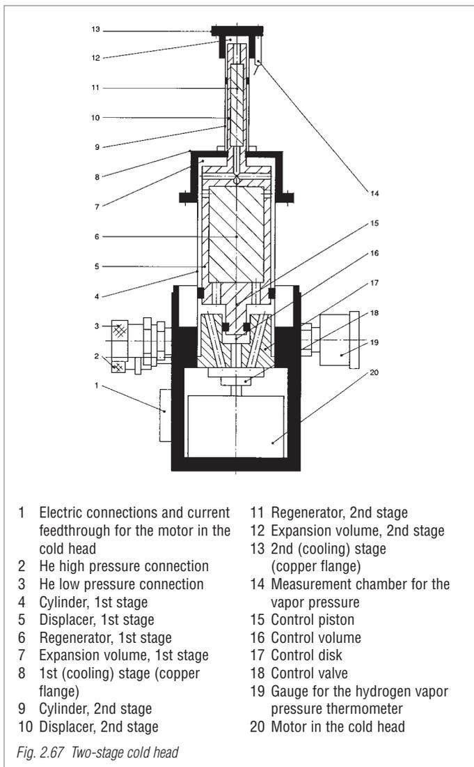
means of a control mechanism with a motor driven control valve (18) with control disk (17) and control holes first the pressure in the control volume (16) is changed which causes the displacers (6) of the first stage and the second stage (11) to move; immediately thereafter the pressure in the entire volume of the cylinder is equalized by the control mechanism. The cold head is linked via flexible pressure lines to the compressor.
