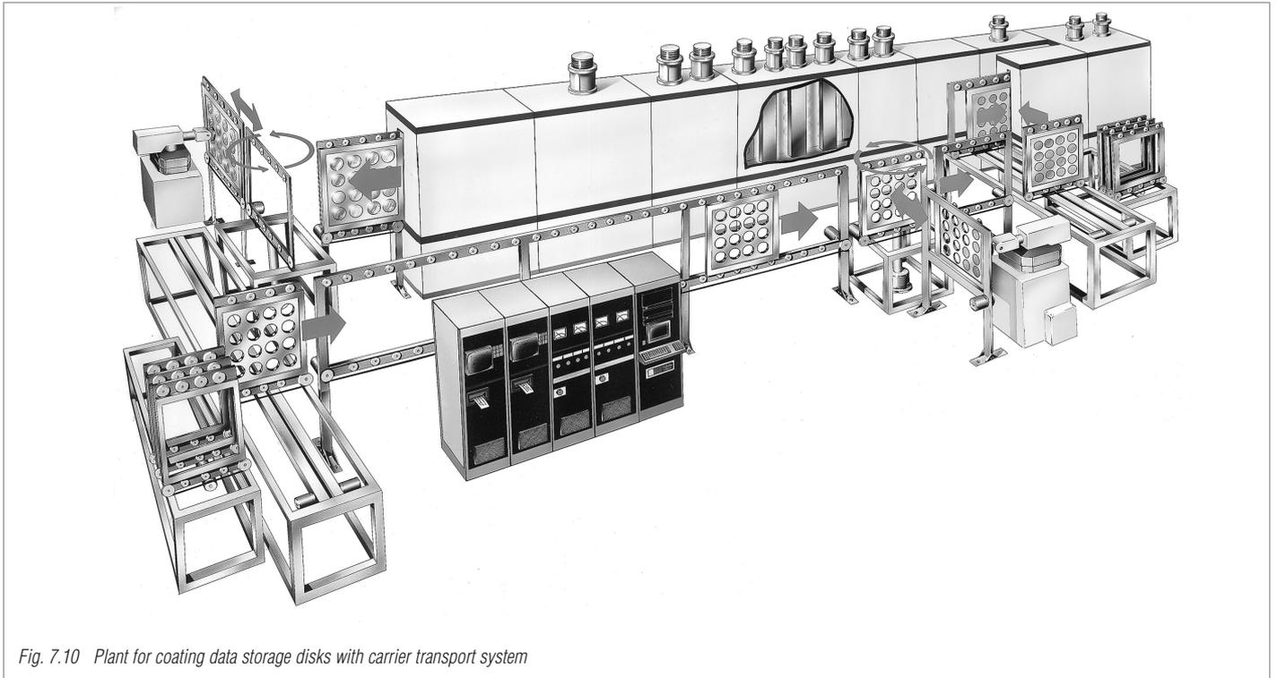
Fig. 7.10 Plant for coating data storage disks with carrier transport system
