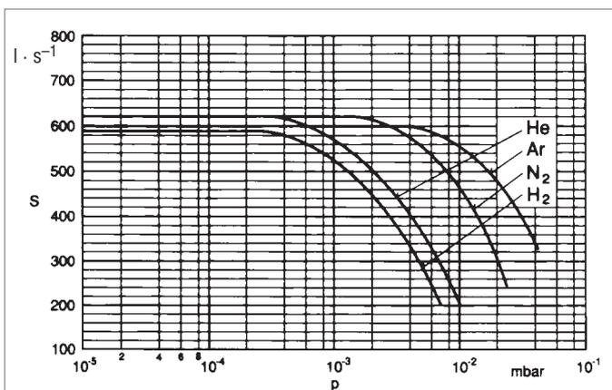
Fig. 2.54 Pumping speed curves of a TURBOVAC 600 for H<sub>2</sub>, He, N<sub>2</sub> and Ar
