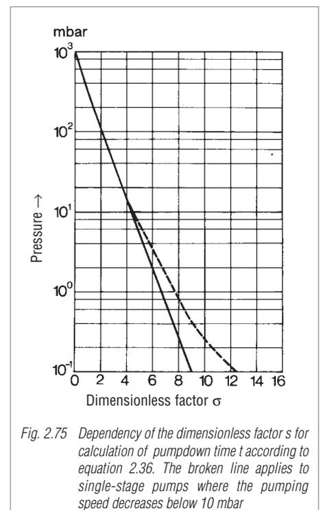
Fig. 2.75 Dependency of the dimensionless factor  $\sigma$  for calculation of pumpdown time  $t$  according to equation 2.36. The broken line applies to single-stage pumps where the pumping speed decreases below 10 mbar
