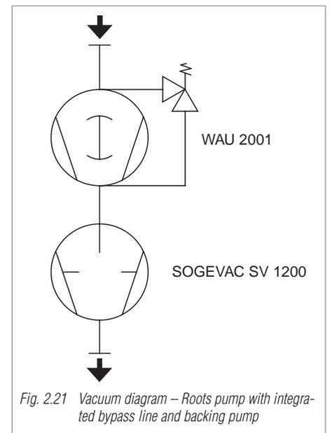
Fig. 2.21 Vacuum diagram – Roots pump with integrated bypass line and backing pump
