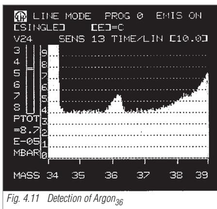
Fig. 4.11 Detection of Argon<sub>36</sub>
