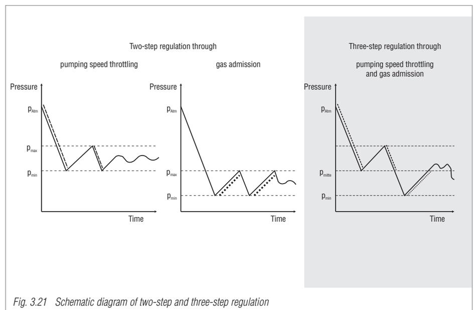
Fig. 3.21 Schematic diagram of two-step and three-step regulation
