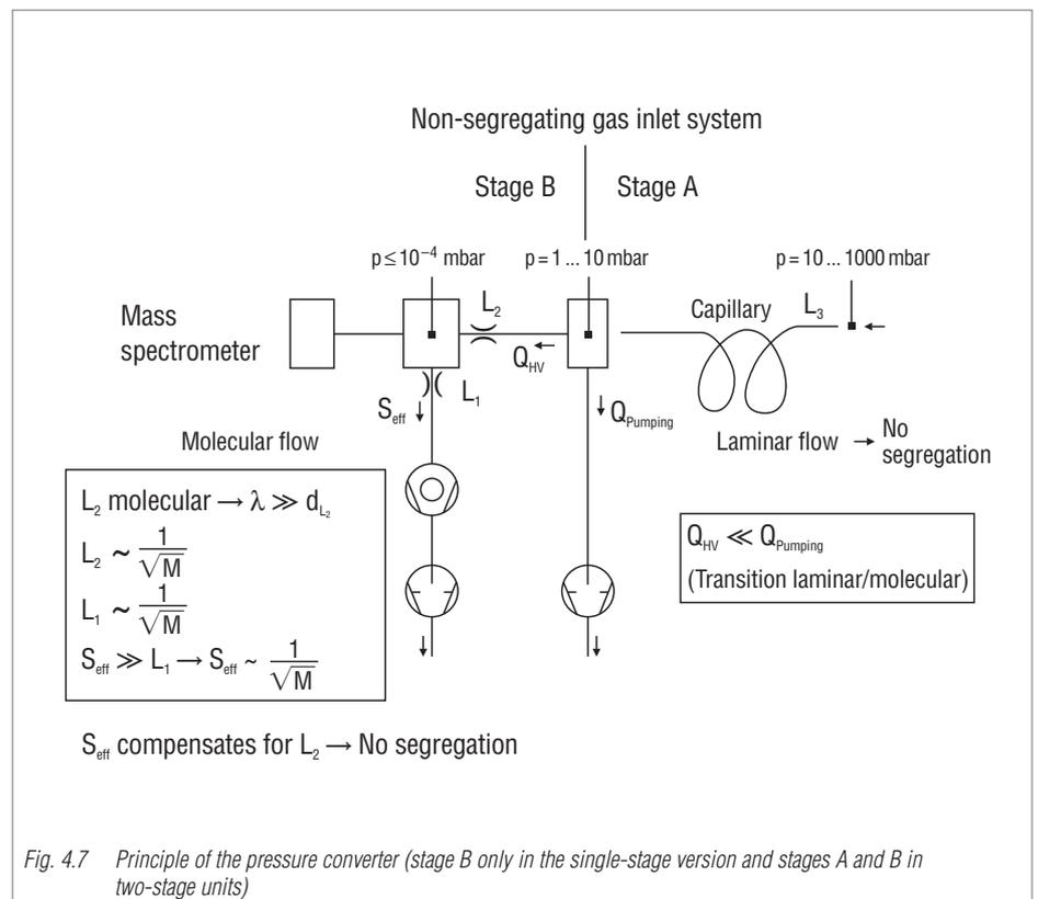
Fig. 4.7 Principle of the pressure converter (stage B only in the single-stage version and stages A and B in two-stage units)
