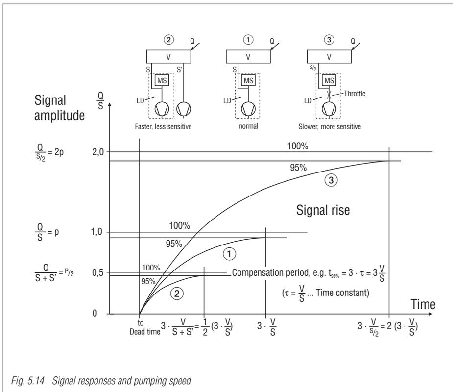
Fig. 5.14 Signal responses and pumping speed
