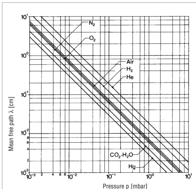
Fig. 9.1: Variation of mean free path λ (cm) with pressure for various gases
