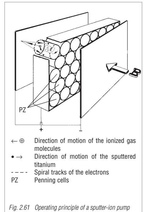
Fig. 2.61 Operating principle of a sputter-ion pump
