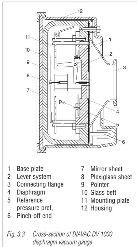
Fig. 3.3 Cross-section of DIAVAC DV 1000 diaphragm vacuum gauge
