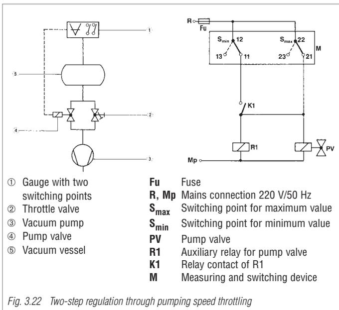
Fig. 3.22 Two-step regulation through pumping speed throttling
