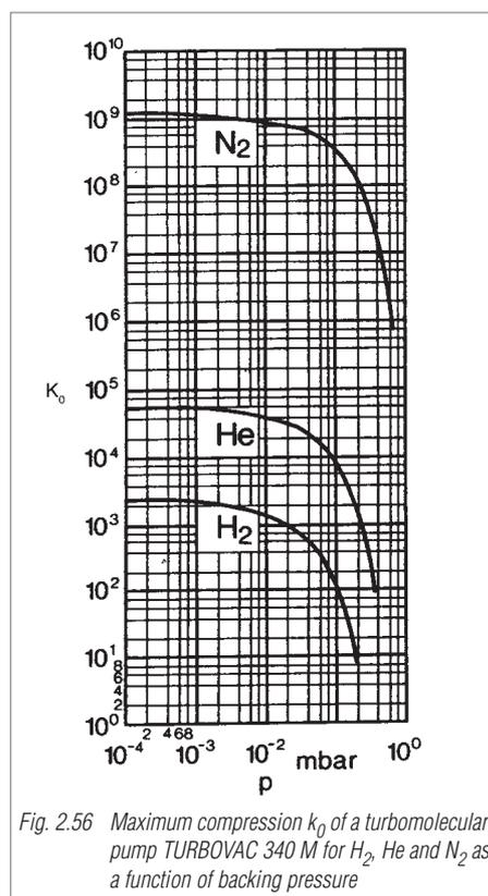
Fig. 2.56 Maximum compression  $k_0$  of a turbomolecular pump TURBOVAC 340 M for H<sub>2</sub>, He and N<sub>2</sub> as a function of backing pressure
