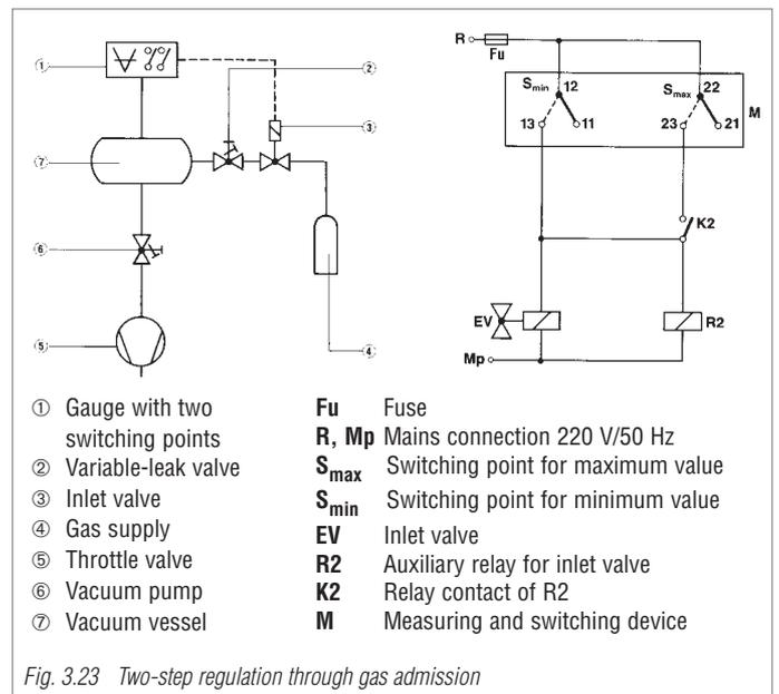
Fig. 3.23 Two-step regulation through gas admission
