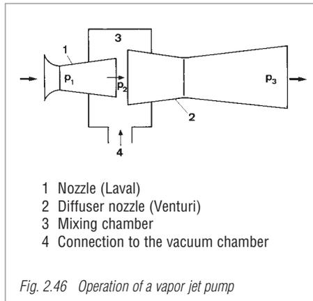
Fig. 2.46 Operation of a vapor jet pump
