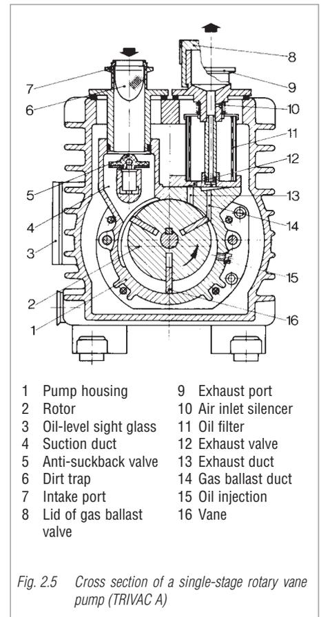
both cases the vanes are forced outwards by the centrifugal forces without the use of springs. At low ambient temperatures this possibly requires the use of a thinner oil. The A-Series is lubricated through the arising pressure difference whereas the B-Series pumps have a geared oil pump for pressure lubrication. The TRIVAC B-Series is equipped with a particularly reliable anti-suckback valve; a horizontal or vertical
