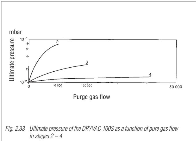
Fig. 2.33 Ultimate pressure of the DRYVAC 100S as a function of pure gas flow in stages 2 – 4
