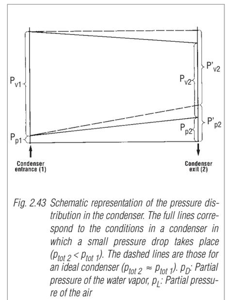
of the condenser, the water vapor partial pressure  $p_{v2}$  lies more or less above the saturation pressure  $p_S$  which corresponds to the temperature of the refrigerant. (By cooling with water at 12 °C,  $p_S$  would be 15 mbar (see Table XIII in Section 9)). Correspondingly, the partial air pressure  $p_{p2}$  that prevails at the condenser exit also varies. With a large condenser,
