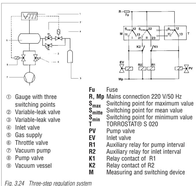
Fig. 3.24 Three-step regulation system
