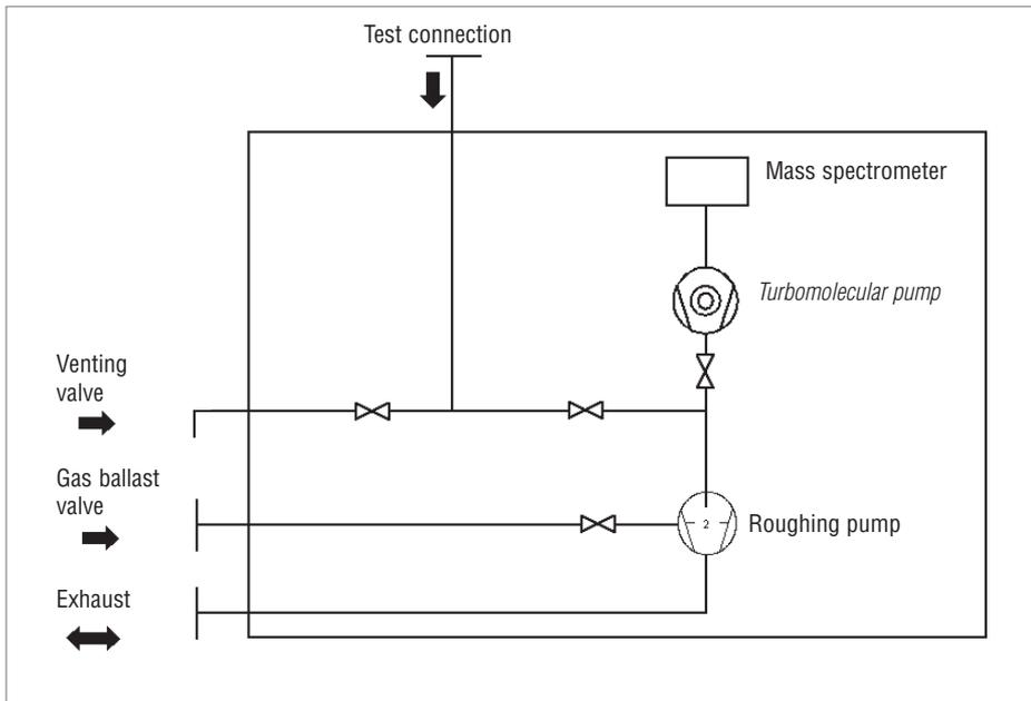
Fig. 5.7 Correct set-up for a MSLD
