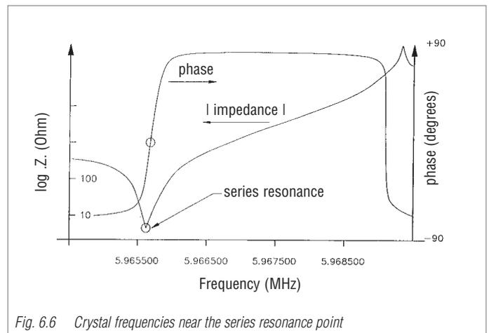
Fig. 6.6 Crystal frequencies near the series resonance point
