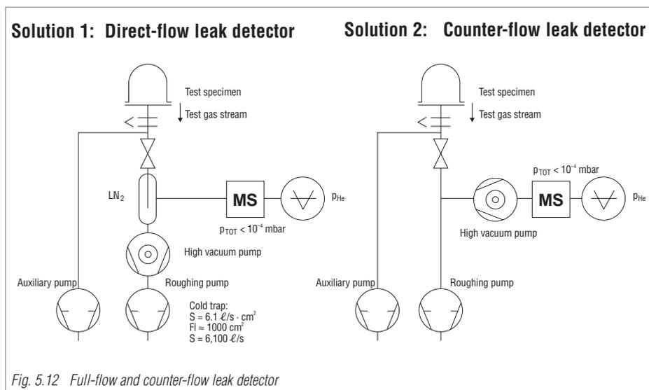
Fig. 5.12 Full-flow and counter-flow leak detector
