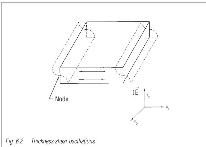
Fig. 6.2 Thickness shear oscillations
