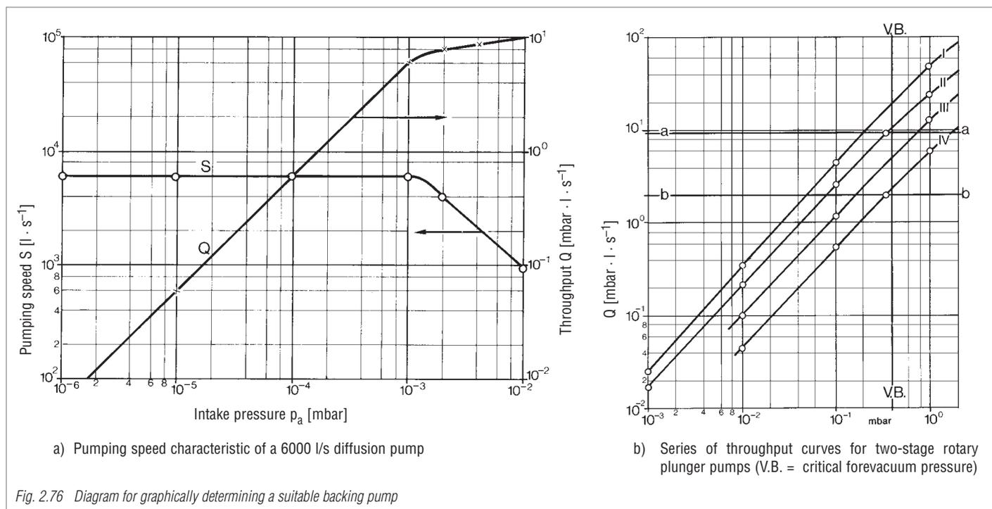
Fig. 2.76 Diagram for graphically determining a suitable backing pump
