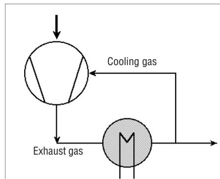
Fig. 2.37 Circulation of the cold gas in the “ALL-ex” with cooler / condenser
