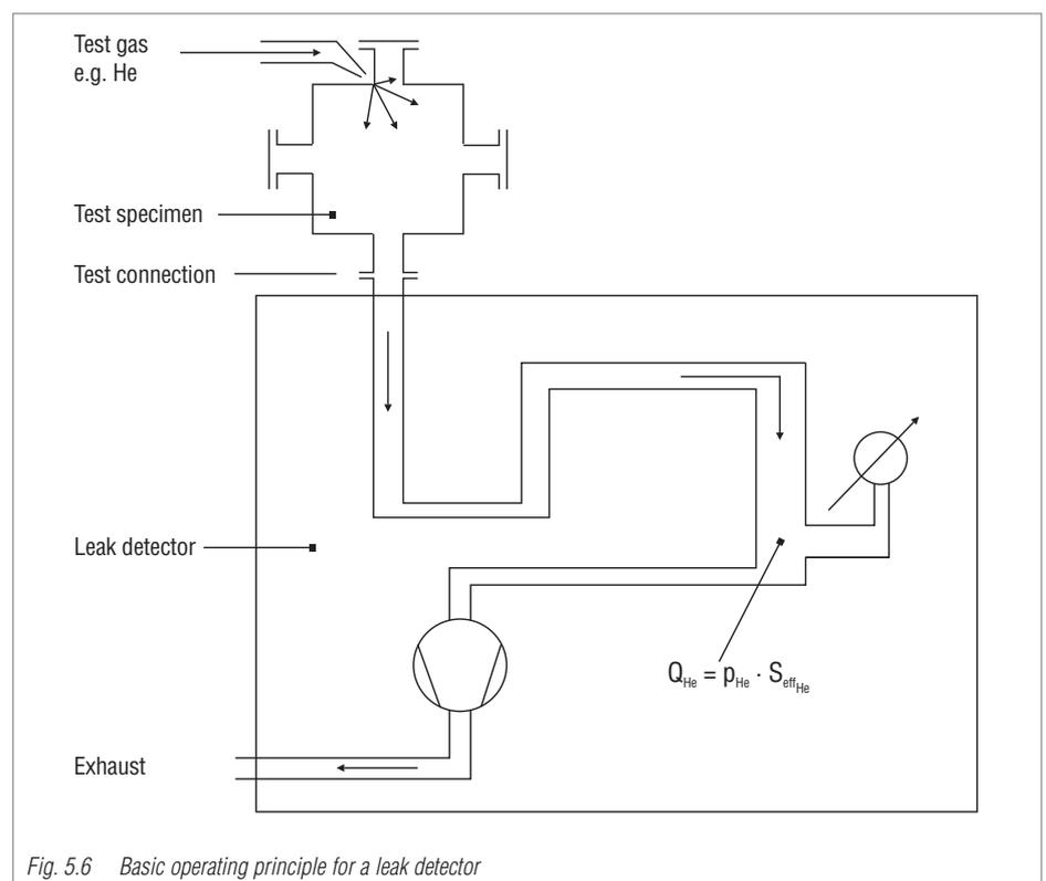
Fig. 5.6 Basic operating principle for a leak detector
