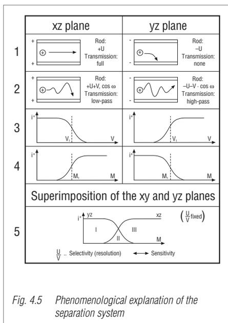
Fig. 4.5 Phenomenological explanation of the separation system
