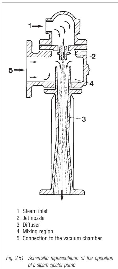
especially recommended for pumping laboratory distillation apparatus and similar plants when the pressure from a simple water jet pump is insufficient. In this instance, the use of rotary pumps would not be economical.
