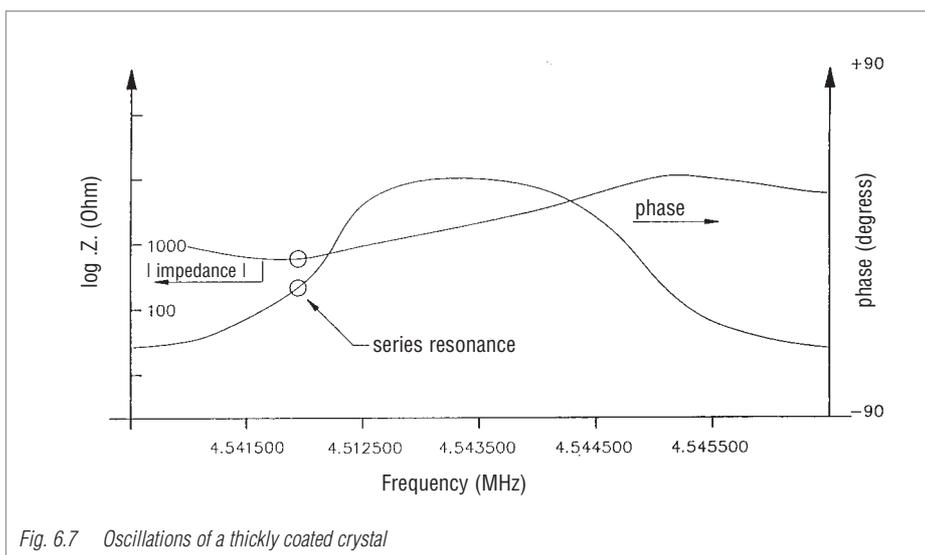
Fig. 6.7 Oscillations of a thickly coated crystal
