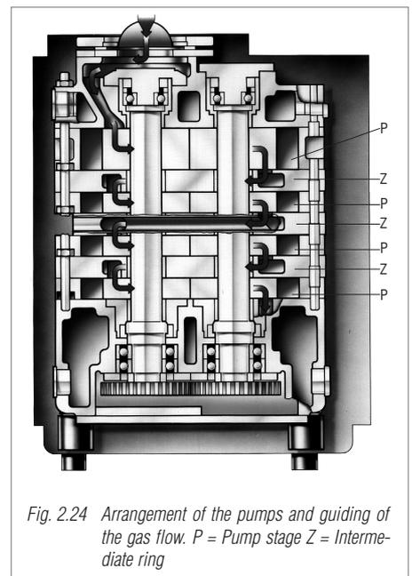
pressure difference of the particular pump. This ensures that the Roots pump is not overloaded and that it may be operated in any pressure range. In practice this means that the Roots pump can be switched on, together with the backing pump, at atmospheric pressure. In the process any pressure increases will not adversely affect combined operation, i.e. the Roots pump is not switched off in such circumstances.
