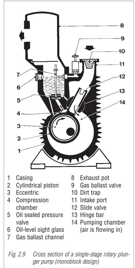
Fig. 2.9 Cross section of a single-stage rotary plunger pump (monoblock design)
