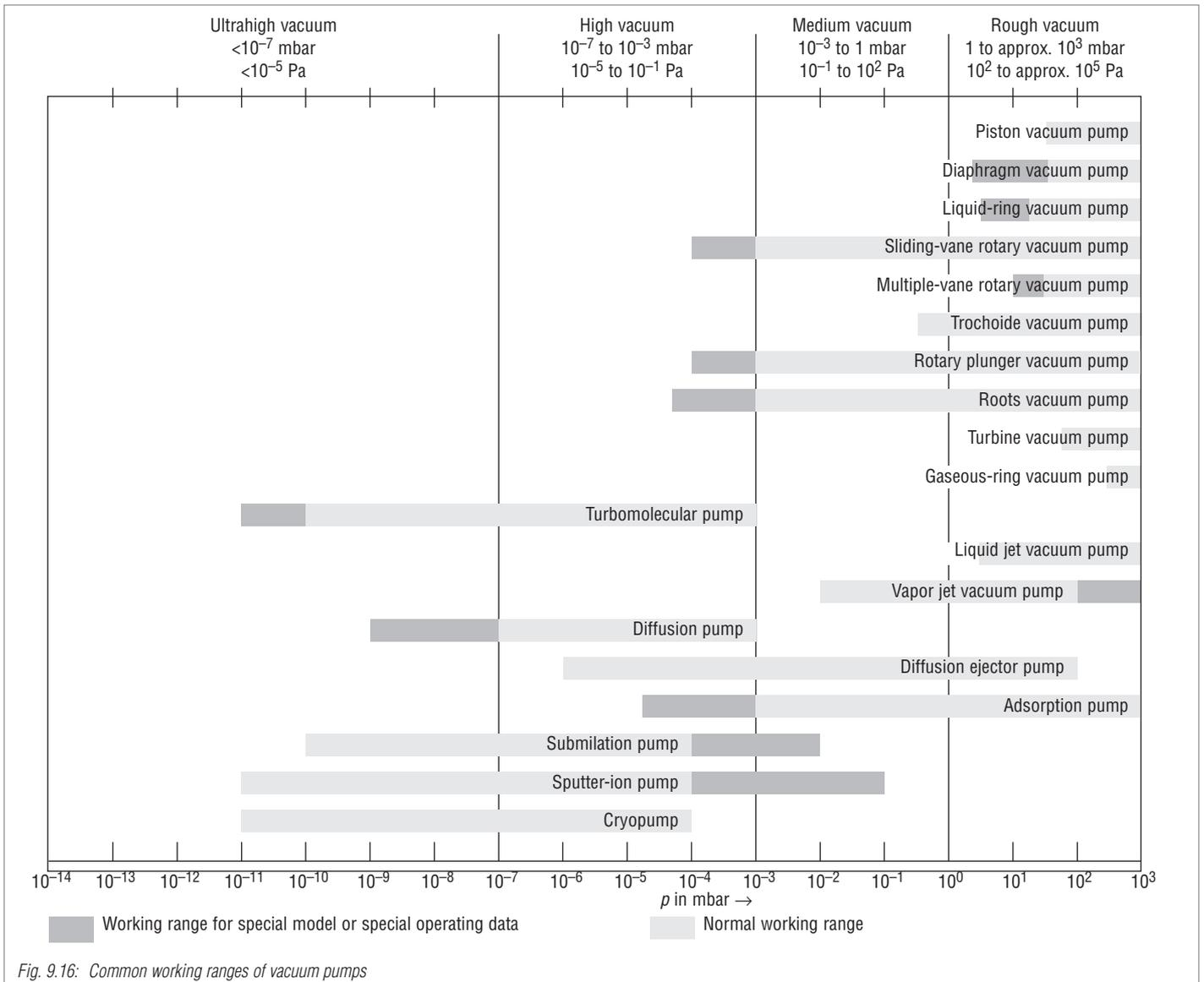
Fig. 9.16: Common working ranges of vacuum pumps
