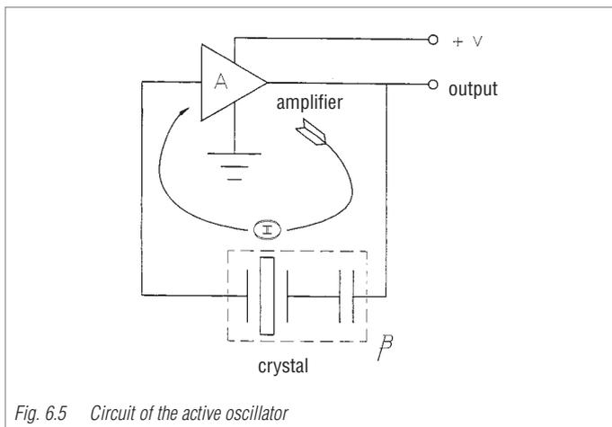
Fig. 6.5 Circuit of the active oscillator
