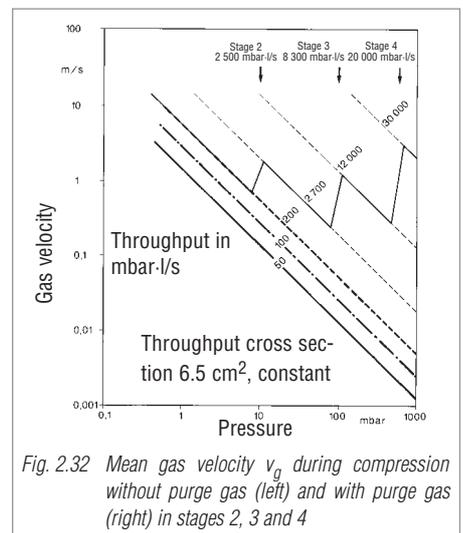
Fig. 2.32 Mean gas velocity  $v_g$  during compression without purge gas (left) and with purge gas (right) in stages 2, 3 and 4
