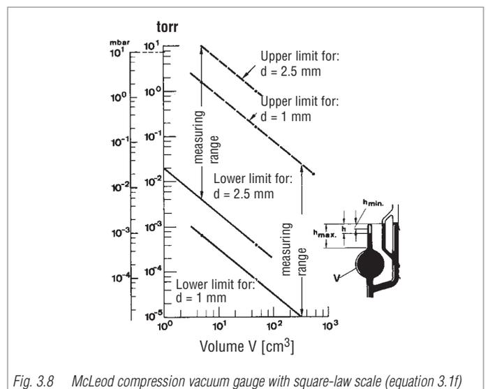
Fig. 3.8 McLeod compression vacuum gauge with square-law scale (equation 3.1f)
