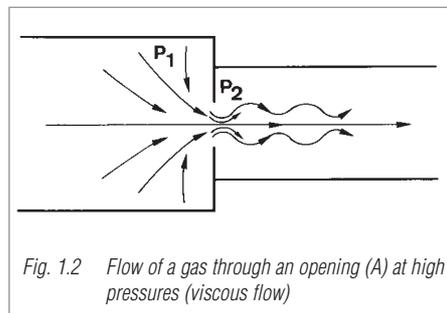
Fig. 1.2 Flow of a gas through an opening (A) at high pressures (viscous flow)
