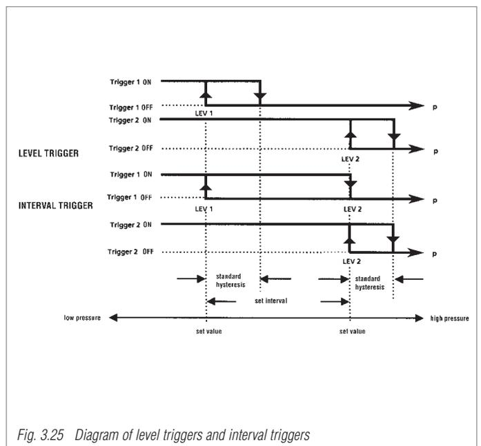
Fig. 3.25 Diagram of level triggers and interval triggers
