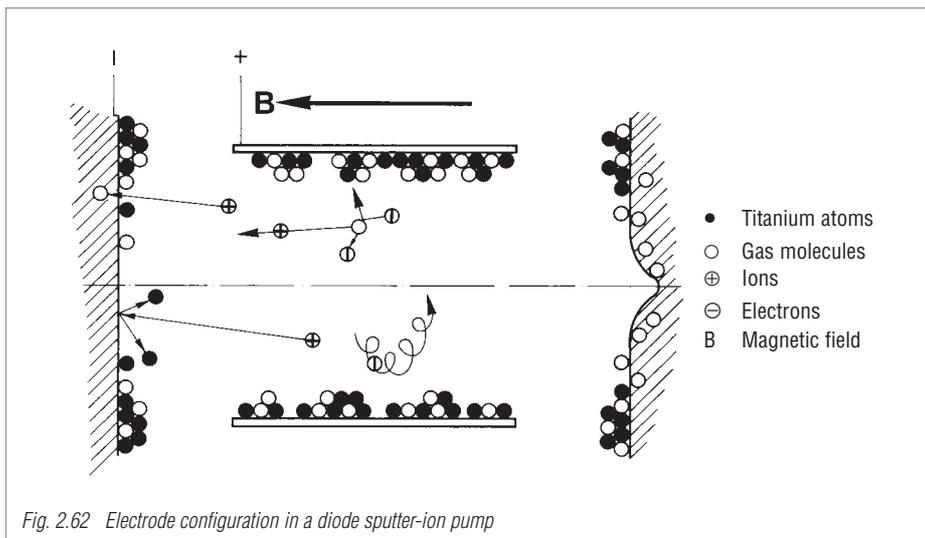
Fig. 2.62 Electrode configuration in a diode sputter-ion pump
