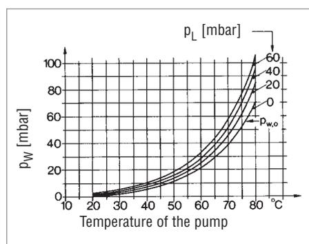
Fig. 2.16 Partial pressure  $p_W$  of water vapor that can be pumped with the gas ballast valve open without condensation in the pump, as a function of the pump temperature for various partial pressures  $p_L$  of air. The lowest curve corresponds to the water vapor tolerance  $p_{W,0}$  of the pump
