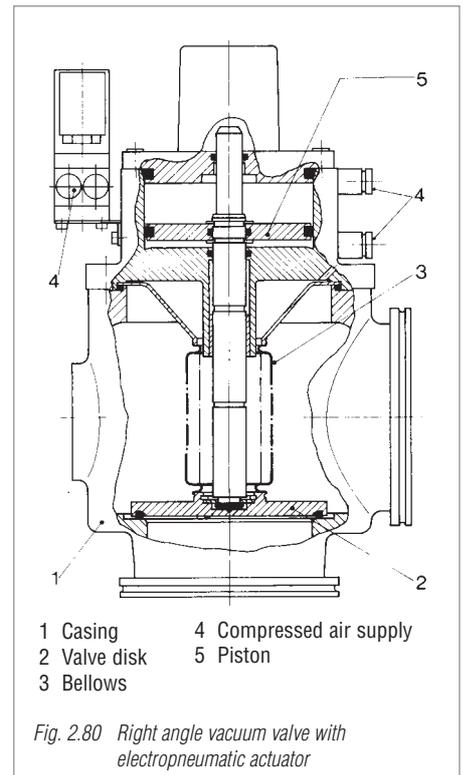
used for highly stringent demands. Their leakage rate is also about  $10^{-9}$  mbar · l/s. However, a special case is the pendulum-type gate valve. Despite its grease-covered seal, the leak rate between vacuum and external atmosphere is virtually the same as for bellows-sealed valves because when the valve is in operation the shaft carries out only a rotary motion so that no gas molecules are transferred into the vacuum. Pendulum-type gate valves are not manufactured by LEYBOLD.
