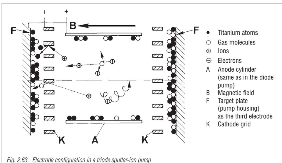
Fig. 2.63 Electrode configuration in a triode sputter-ion pump
