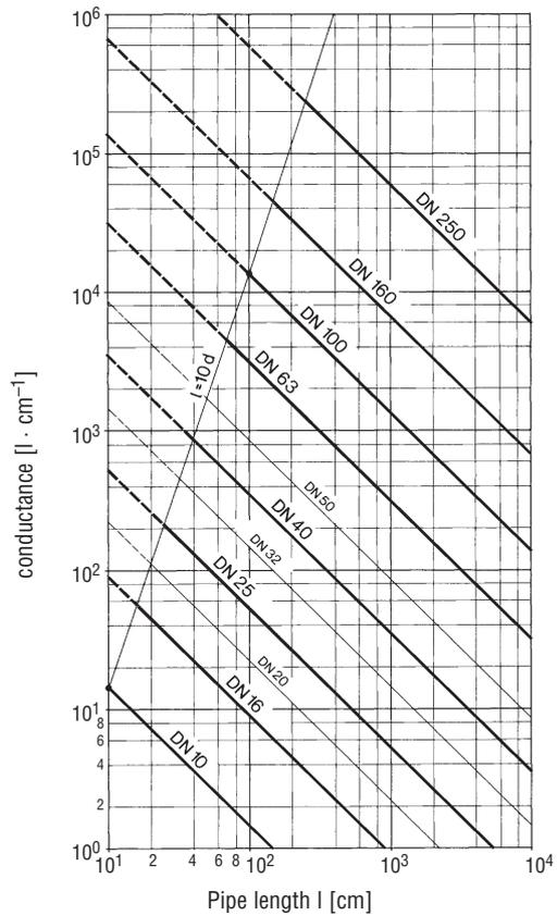
Fig. 9.5: Conductance values for piping of commonly used nominal width with circular cross-section for laminar flow ( $p = 1$  mbar) according to equation 53a. (Thick lines refer to preferred DN) Flow medium: air ( $d, l$  in cm!)
