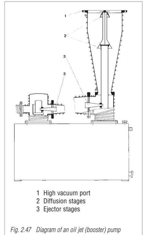
Fig. 2.47 Diagram of an oil jet (booster) pump
