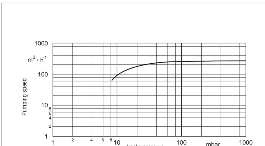
Fig. 2.39 Pumping speed characteristic of an ALL-ex” 250
