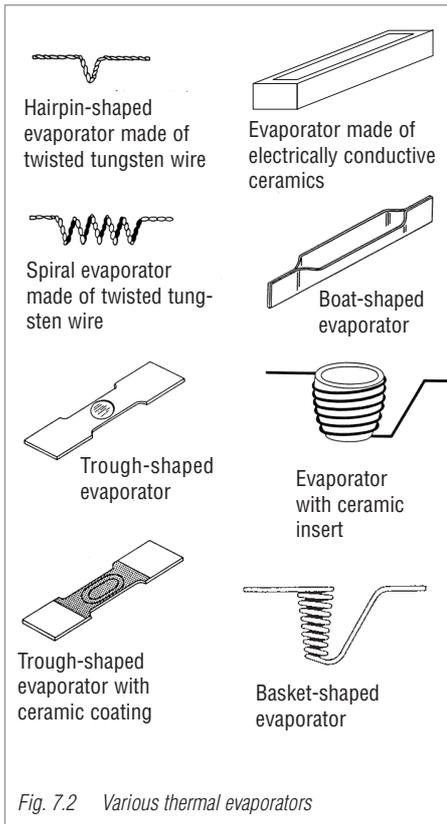
Fig. 7.2 Various thermal evaporators
