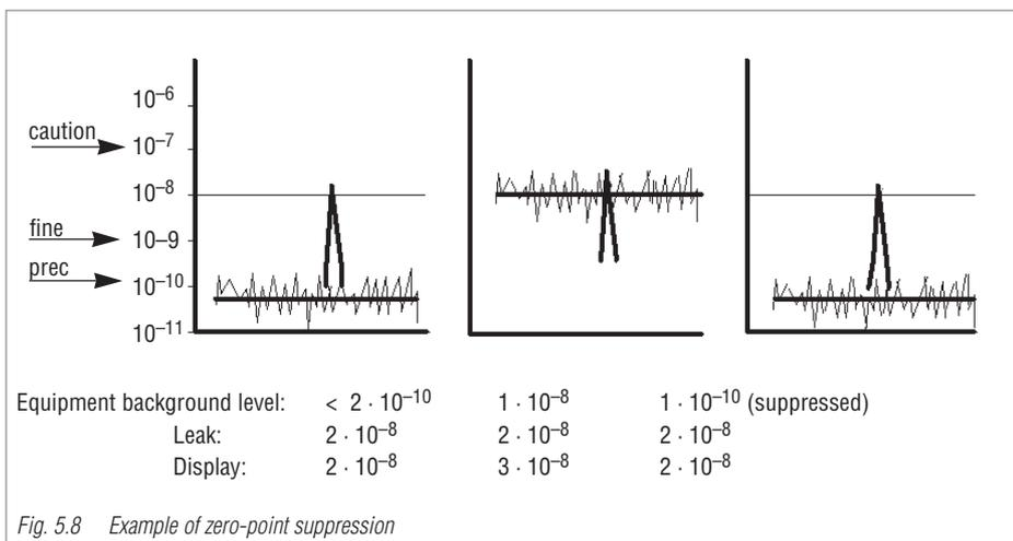
Fig. 5.8 Example of zero-point suppression
