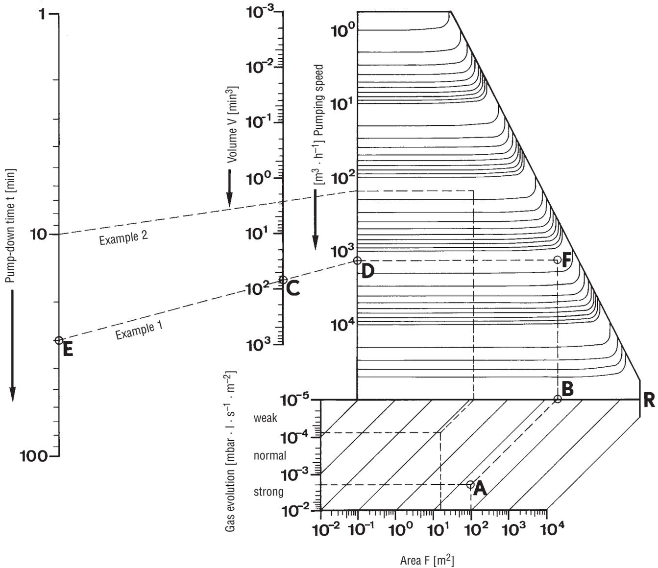
The nomogram indicates the relationship between the nominal pumping speed of the pump, the chamber volume, size and nature of the inner surface as well as the time required to reduce the pressure from 10 mbar to 10<sup>-3</sup> mbar.
