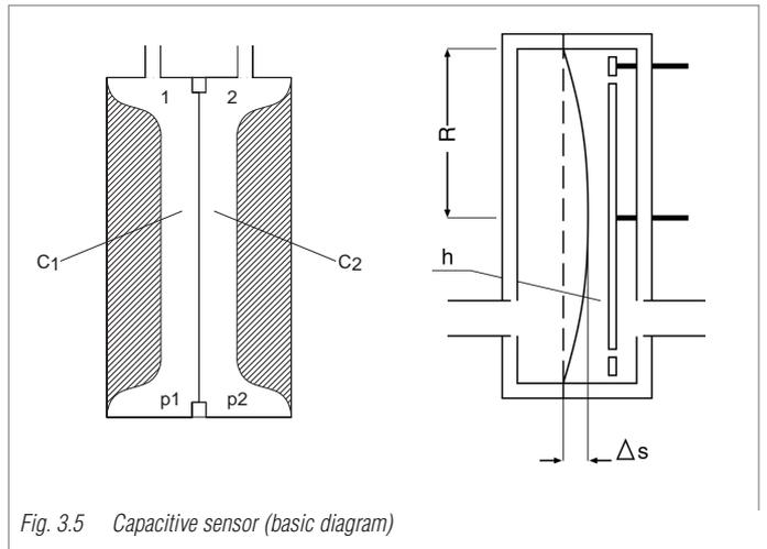
**3.2.2.4 Capacitance diaphragm gauges**
