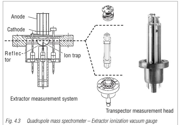
Fig. 4.3 Quadrupole mass spectrometer – Extractor ionization vacuum gauge
