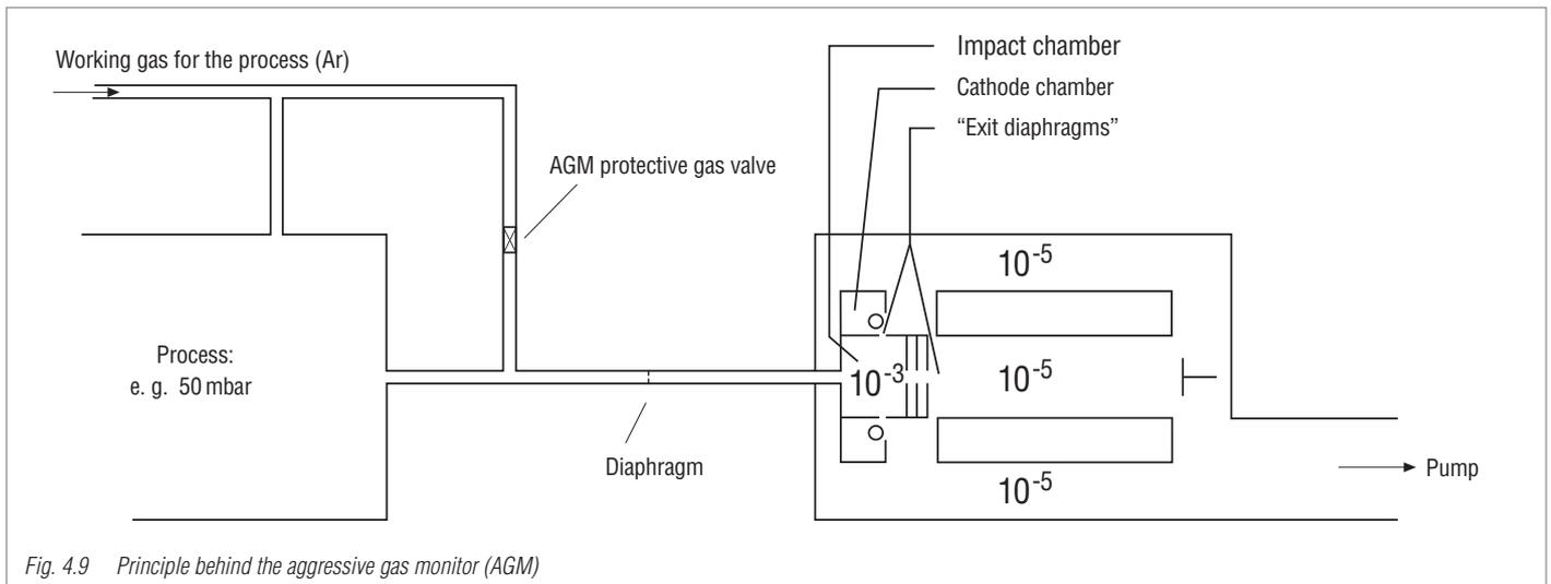
Fig. 4.9 Principle behind the aggressive gas monitor (AGM)
