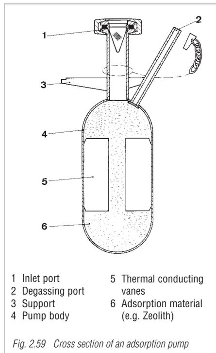
Fig. 2.59 Cross section of an adsorption pump
