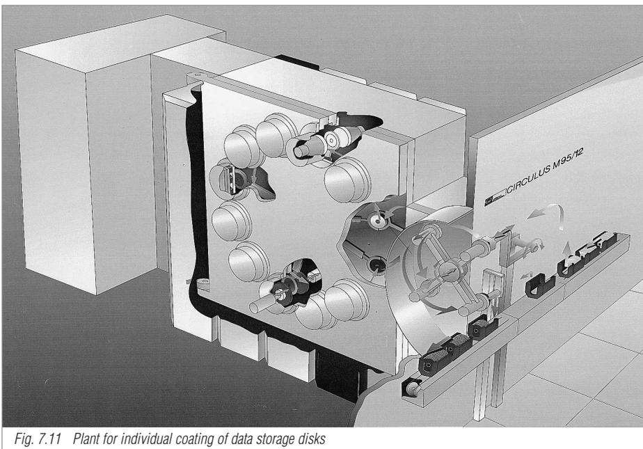
Fig. 7.11 Plant for individual coating of data storage disks
