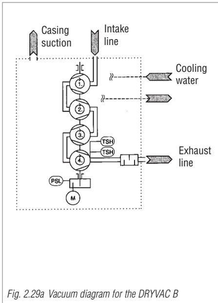
Fig. 2.29a Vacuum diagram for the DRYVAC B
