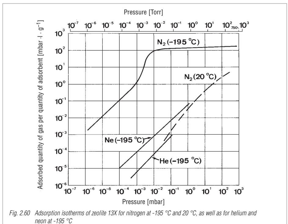
Fig. 2.60 Adsorption isotherms of zeolite 13X for nitrogen at -195 °C and 20 °C, as well as for helium and neon at -195 °C
