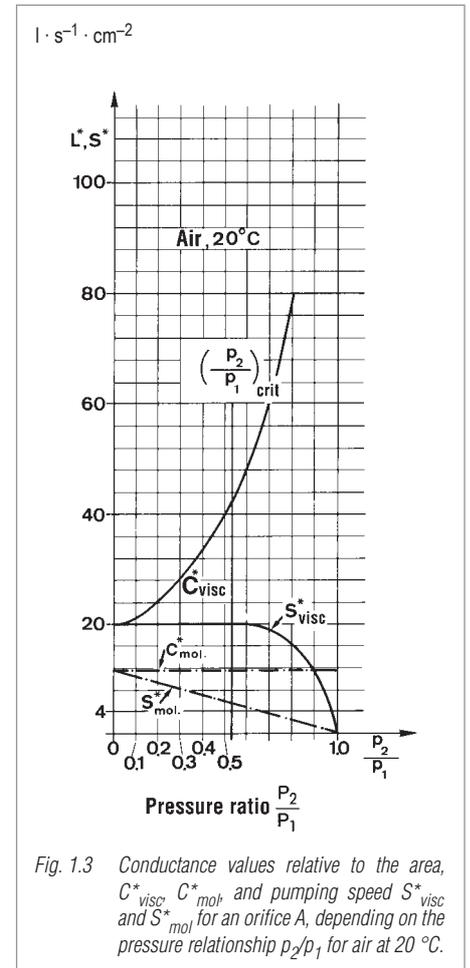
Fig. 1.3 Conductance values relative to the area,  $C^*_{\text{visc}}$ ,  $C^*_{\text{mol}}$  and pumping speed  $S^*_{\text{visc}}$  and  $S^*_{\text{mol}}$  for an orifice A, depending on the pressure relationship  $p_2/p_1$  for air at 20 °C.
