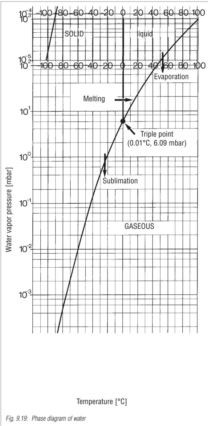
Fig. 9.19: Phase diagram of water
