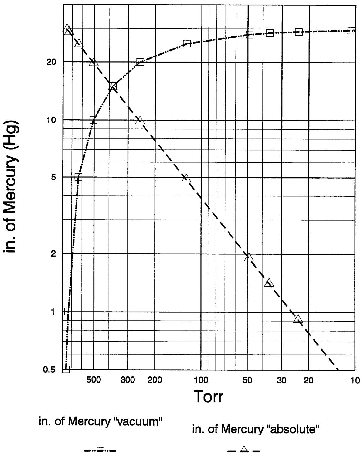
Figure 25 - Conversion graph: Torr to in Hg
