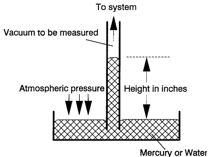
**Figure 2 - Representation of a gauge vacuum measurement**
