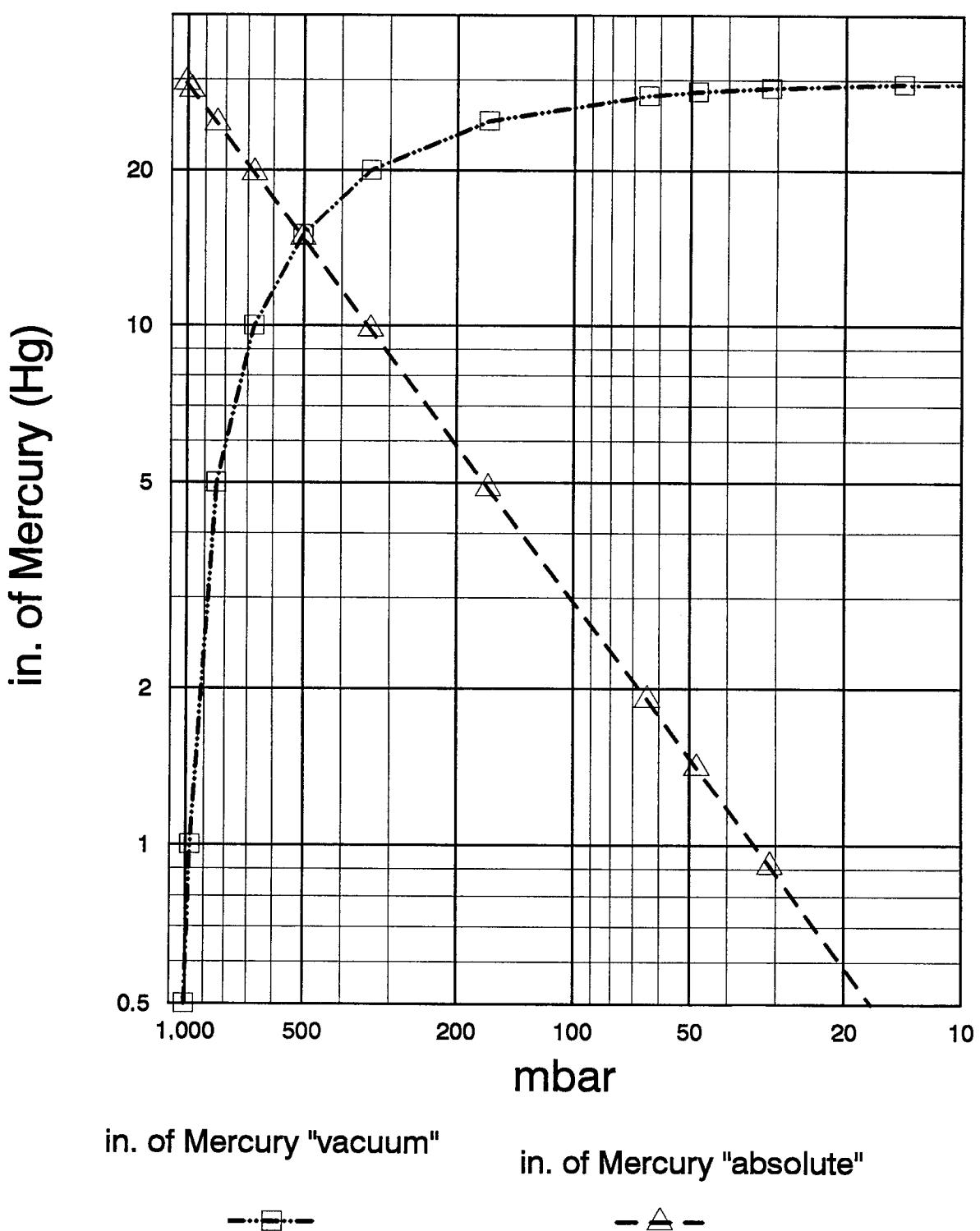
Figure 8 - Conversion graph: mbar to in Hg
