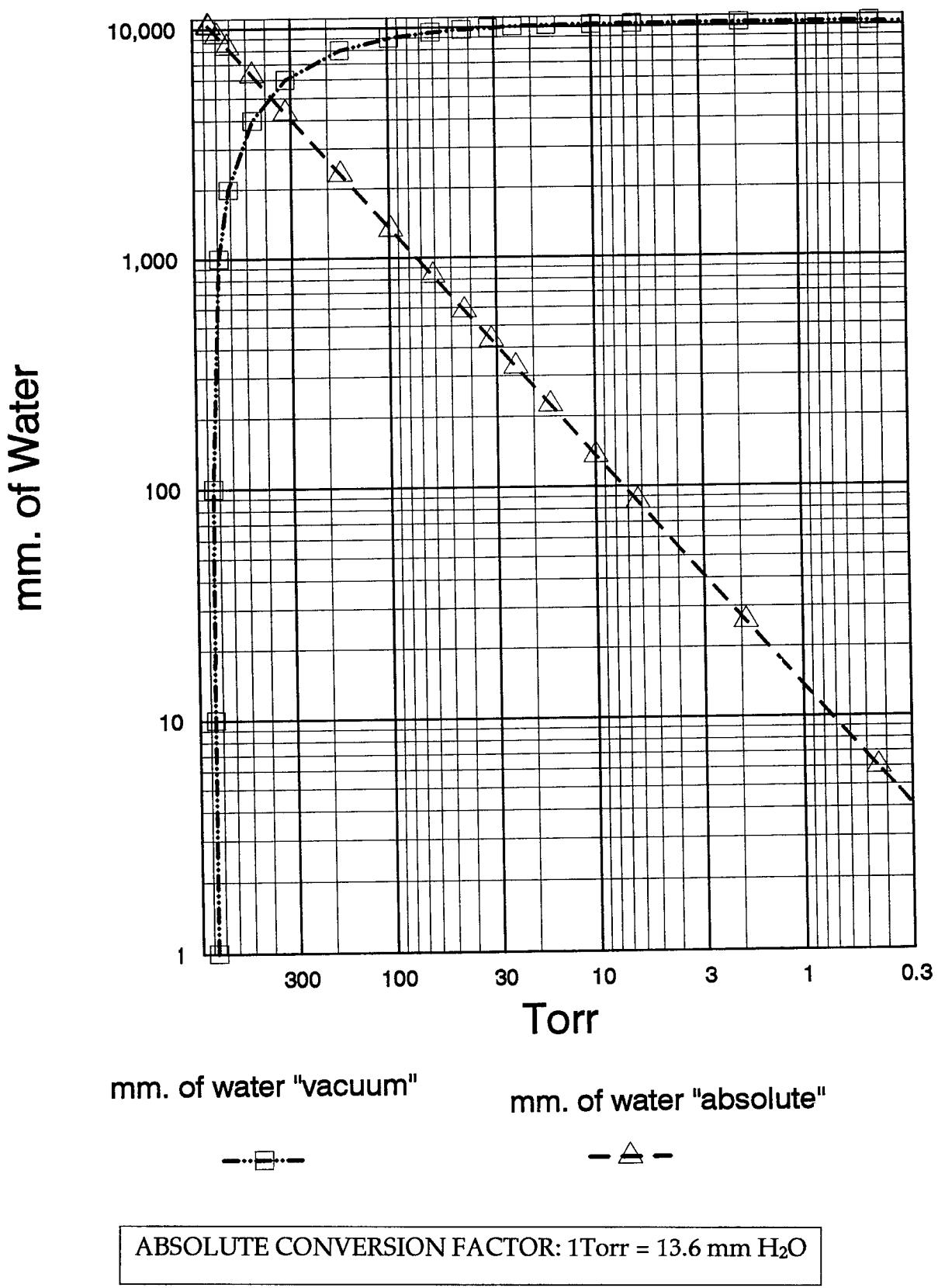
Figure 24 - Conversion graph: Torr to mm H<sub>2</sub>O
