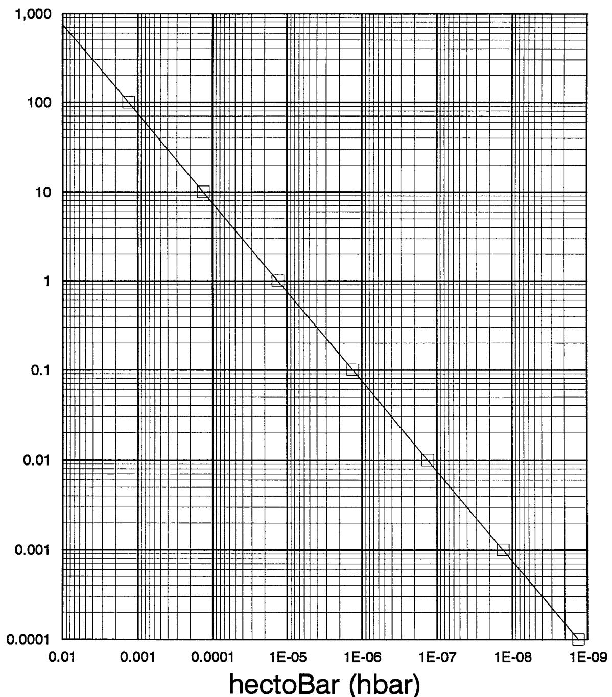
Figure 31 - Conversion graph: (1000 to  $1 \times 10^{-4}$ ) Torr to hbar
