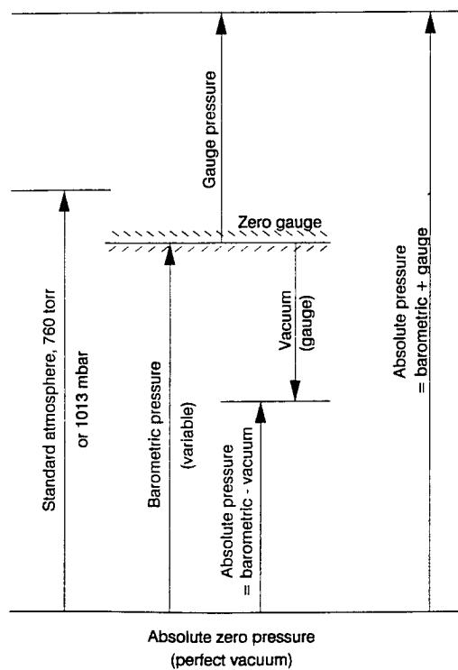
Figure 1 - Representation of vacuum pressure measurement scales
