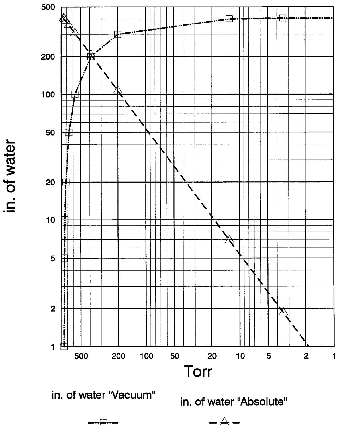
Figure 23 - Conversion graph: Torr to in H<sub>2</sub>O
